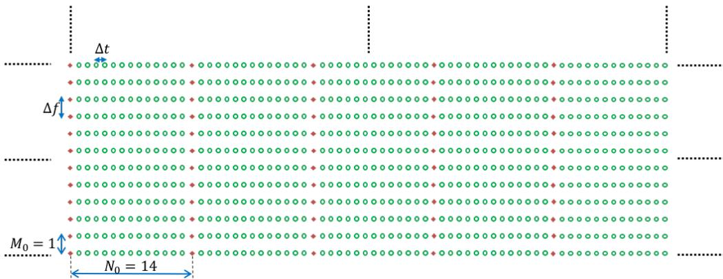
**Figure 2: Time-frequency reference signal grid example.**
