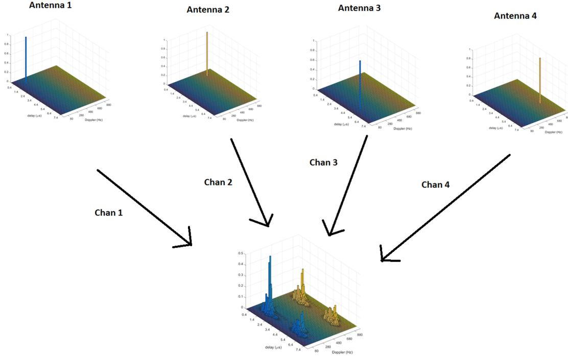
**Figure 1: Reference signals multiplexed in the delay-Doppler domain**
