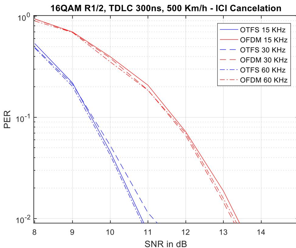
**Figure 5: PER for 1x1 OTFS vs OFDM for varying subcarrier spacing**
