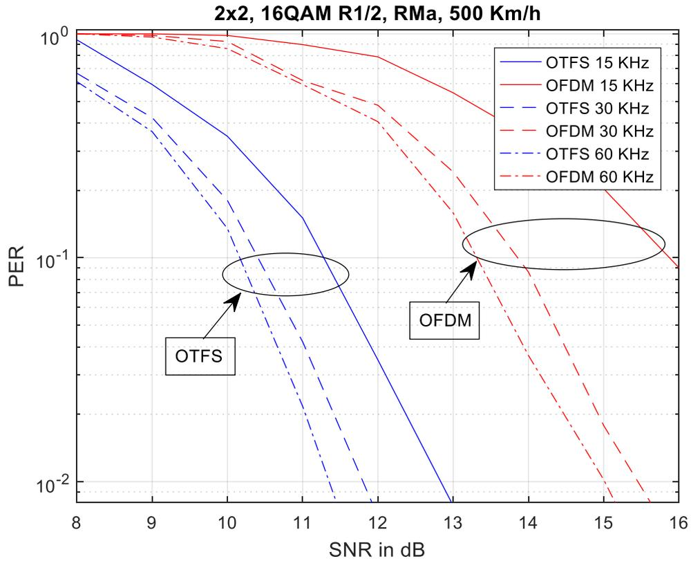
**Figure 2: PER for 2x2 OTFS vs OFDM for varying subcarrier spacing.**
