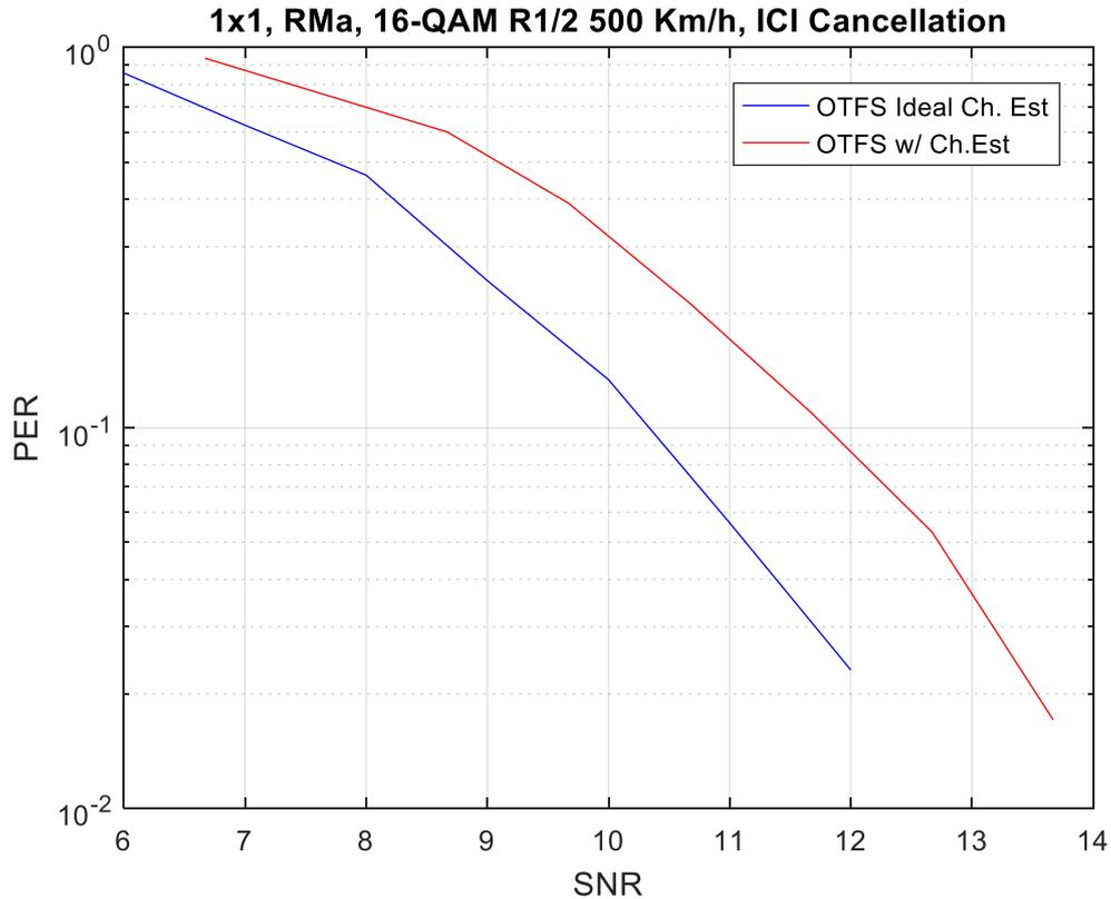
**Figure 6: Comparison of ideal vs pilot based channel estimation**
