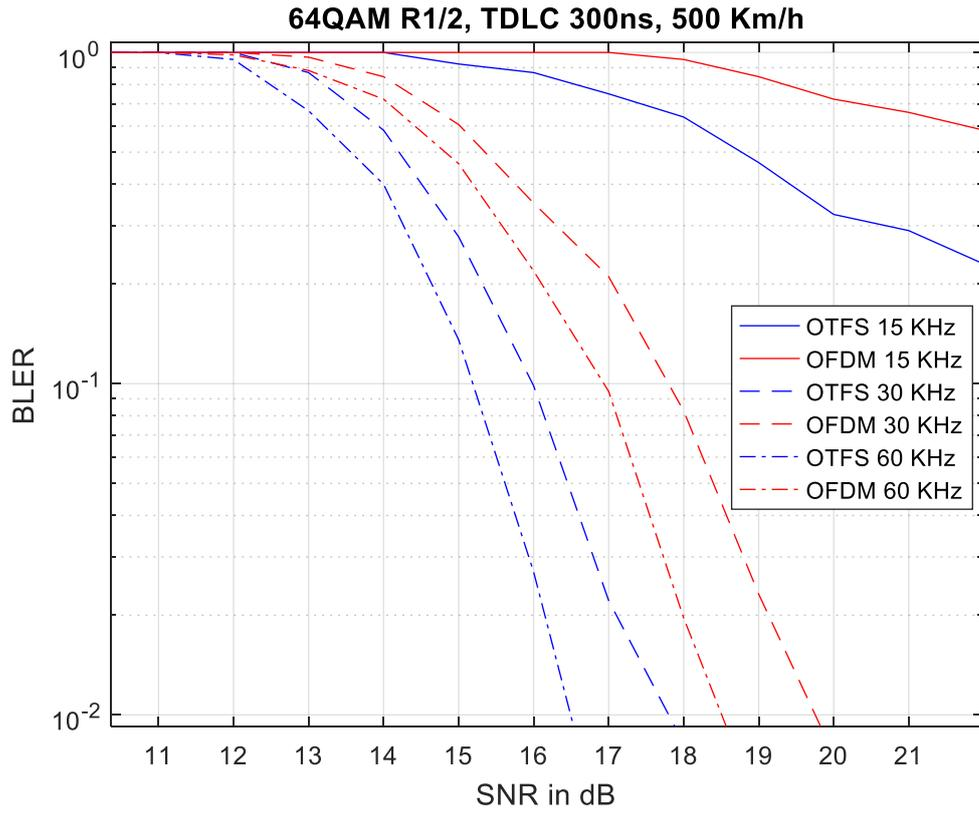
Figure 3: PER for 1x1 OTFS vs OFDM for varying subcarrier spacing
