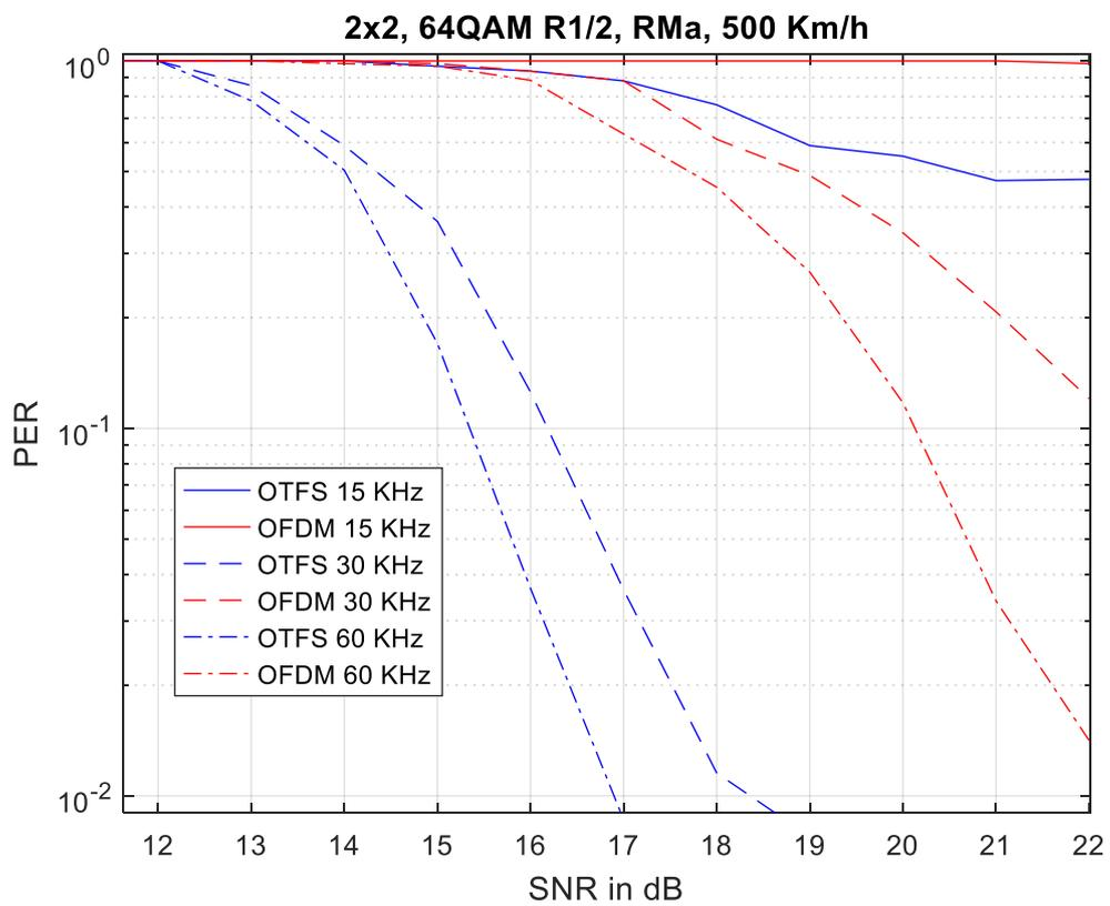
Figure 4: PER for 2x2 OTFS vs OFDM for varying subcarrier spacing
