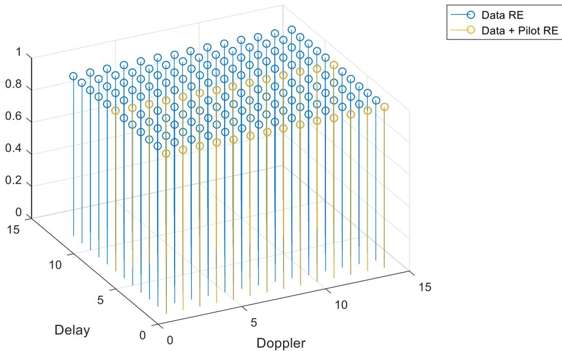
**Figure 7: Data and pilot overlay on one PRB**
